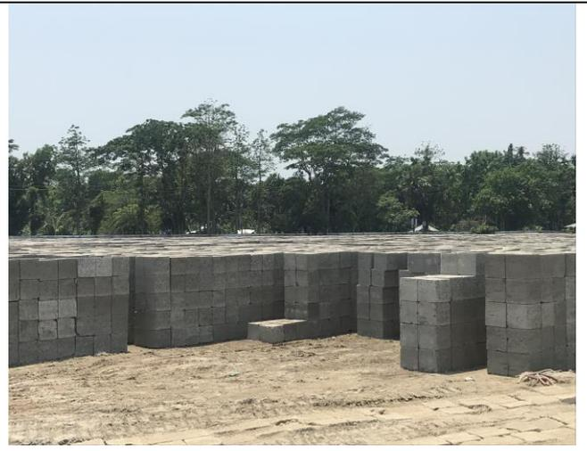
Figure 3-63: Manufactured CC Blocks piled at the permanent storing yard #A2 in Polder 39/2C
